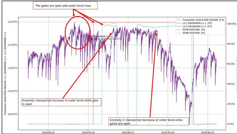
Figure 2. Anomalies detected at the Lockport Powerhouse in June 2018.
